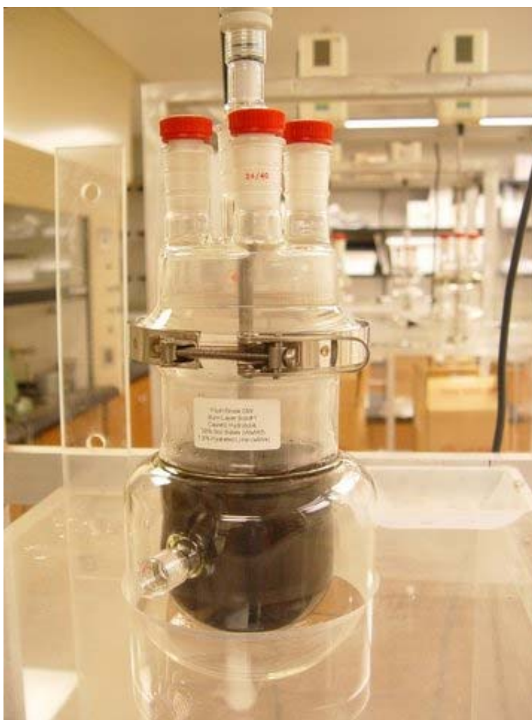
Figure 16. Soil slurry reactor.
